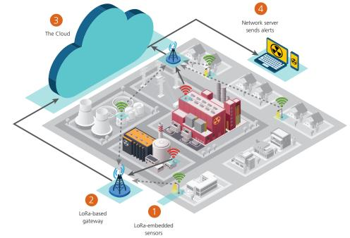
Semtech products used in this application: Sensors Gateway • SX1272/3 • SX1301 • SX1276/7/8/9 All application elements (sensing modules, gateways, servers, software) are available through LoRa Alliance<sup>®</sup> partners.
