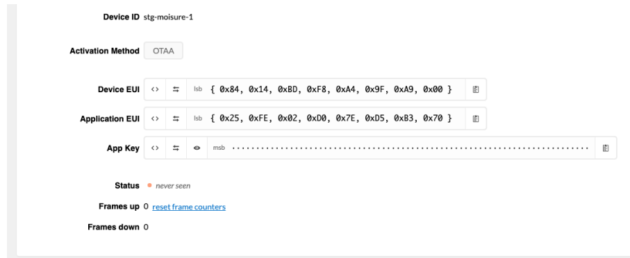
Figure 32: Device details page on TTN showing the Device EUI and Application EUI in the format required
