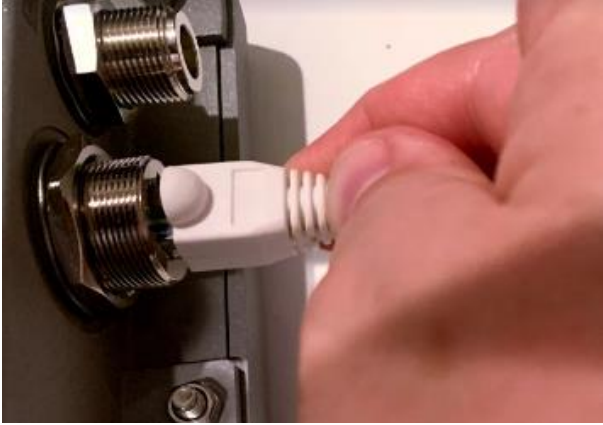
Figure 5: Connecting the Ethernet cable to the gateway
