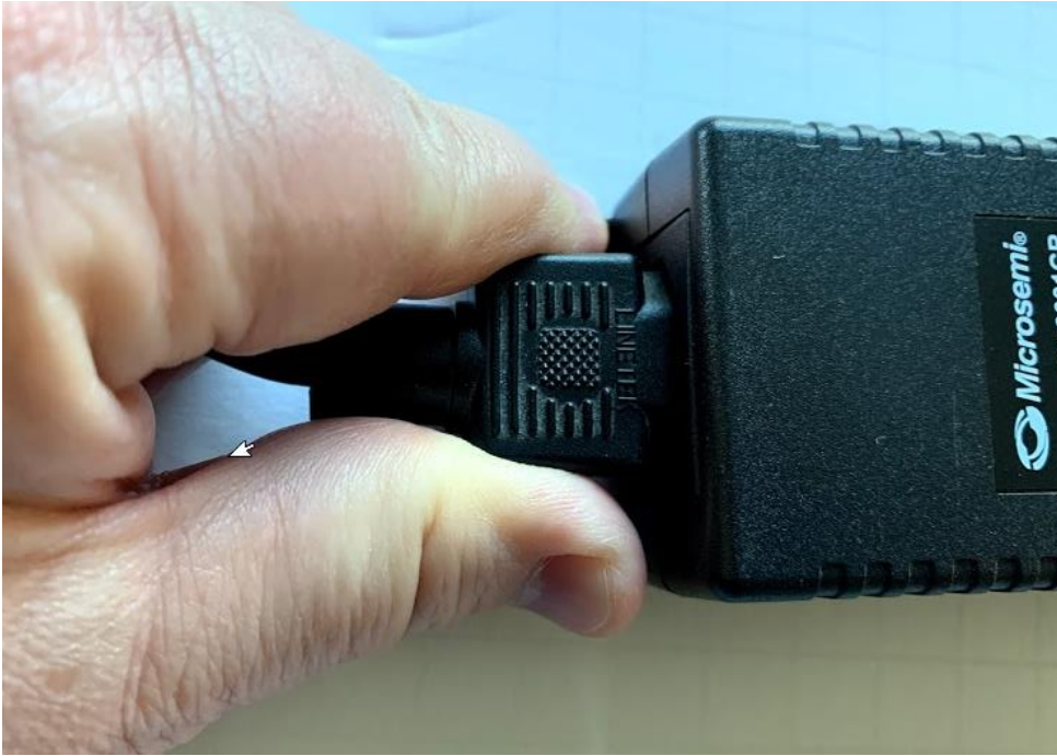
Figure 10: Connecting mains cable to power brick
