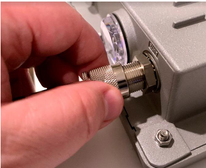
Figure 4: Connecting the LoRa antenna to the gateway
