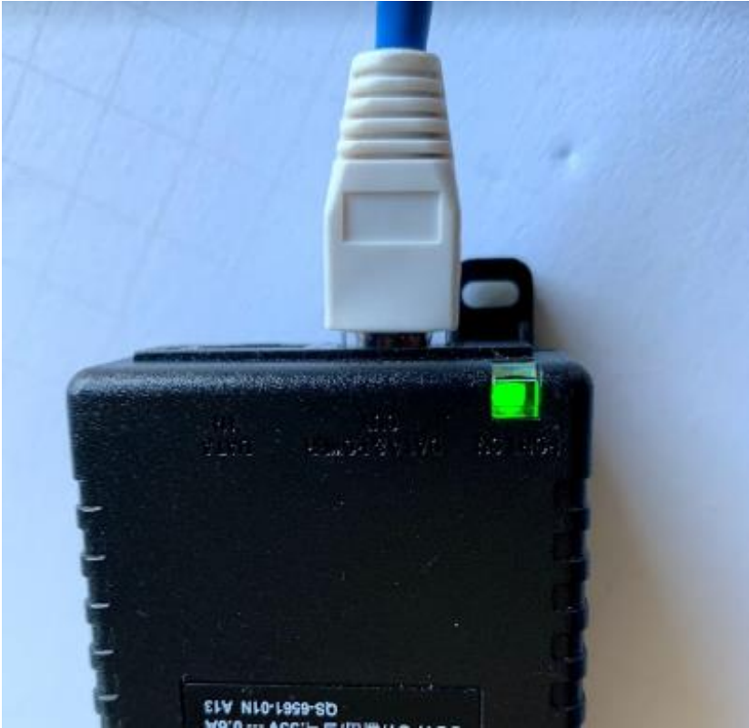
Figure 11: Green LED on Power Brick Means Gateway is Powered
