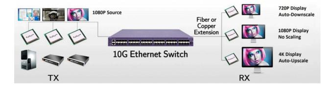
**True seamless switching in n×m signal distribution** – In a matrix-switching environment, switching a display from one source to another typically results in a black screen, frozen frames or other artifacts. With BlueRiver AV Processor's scaling capability integrated into an AV-over-IP platform, truly seamless switching can be achieved where the switching delay is only 1-2 frames and without artifacts, irrespective of the resolution of the switched source.
